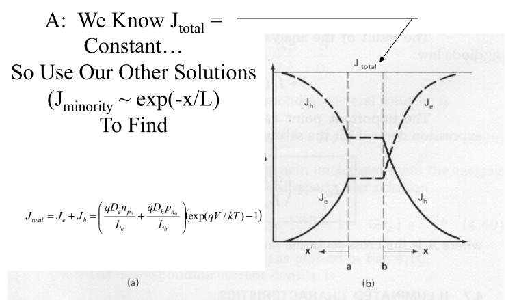
Figure 4.9. (a) Minority-carrier current densities in a p-n junction diode corresponding to Fig. 4.8. (b) Distribution of minority, majority, and total current densities in the diode, neglecting recombination in the depletion region.
