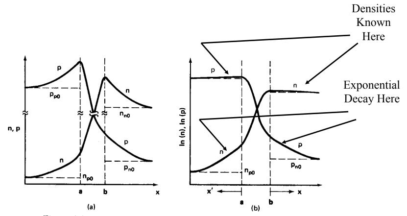
Figure 4.8. (a) Linear plot of the distributions of carriers throughout the p-n junction diode under forward bias. (b) Corresponding semilogarithmic plot. Note the differences with respect to majority carriers.
