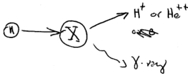
Figure 13.10: Schematic of a neutron-nucleus interaction that leads to the subsequent emission of charged particles.
