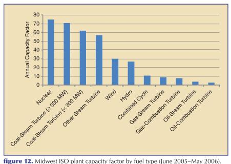
**figure 12.** Midwest ISO plant capacity factor by fuel type (June 2005–May 2006). Adapted from U.S. Department of Energy report *20% Wind by 2030*, July 2008.
