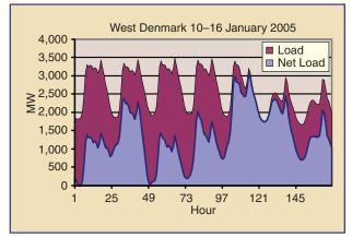
**figure 1.** West Denmark load and net load (load less wind), 10–16 January 2005 (source: Energinet.dk).
