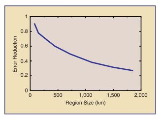
**figure 6.** Decrease of the wind forecast error for aggregated wind power production due to spatial smoothing effects (source: Energy & Meteo Systems).
