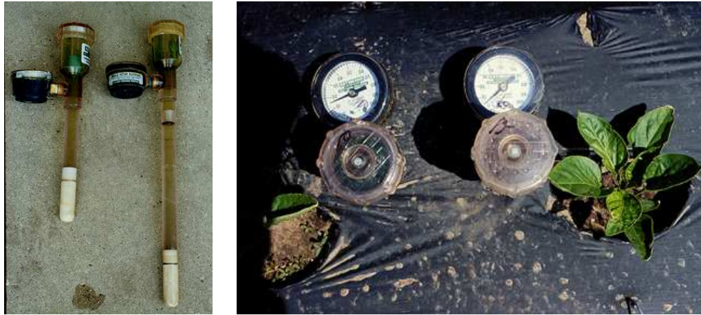
Figure 3.5: Tensiometers are often used to measure suction in unsaturated soils.
