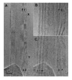
**FIGURE 19.5** HRTEM image of an MWCNT. Note the presence of anomalously large interfringe spacings indicated by arrows. (From Amelinckx S, Lucas A, and Lambin P, (1999), Electron diffraction and microscopy of nanotubes, *Rep. Prog. Phys.* 62(11): 1471–1524. With permission.)
