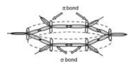
FIGURE 19.1 Basic hexagonal bonding structure for one graphite layer (the *graphene sheet*). Carbon nuclei shown as filled circle, out-of-plane  $\pi$ -bonds represented as delocalized (dotted line), and  $\sigma$ -bonds connect the C nuclei in-plane.
