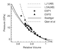
**FIGURE 19.27** Comparison of EOS for graphite using different models with experimental data. (From Qian D, Liu WK, and Ruoff RS, (2001), Mechanics of c60 in nanotubes, *J. Phys. Chem. B.* 105: 10753–10758. With permission of Elsevier Science.)
