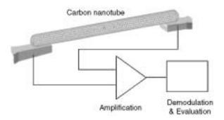
FIGURE 19.38 Carbon nanotube-based sensor.
