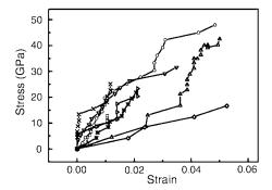
FIGURE 19.6 Eight stress vs. strain curves obtained from the tensile-loading experiments on individual SWCNT bundles. The values of the nominal stress are calculated using the cross-sectional area of the perimeter SWCNTs assuming a thickness of 0.34 nm. (From Yu MF, Files BS, Arepalli S, and Ruoff RS, (2000), Tensile loading of ropes of single-wall carbon nanotubes and their mechanical properties, *Phys. Rev. Lett.* 84(24): 5552–5555. With permission.)
