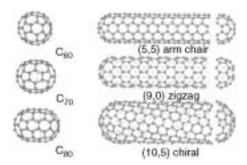
**FIGURE 19.3.** Examples of zigzag, chiral, and armchair nanotubes and their caps corresponding to different types of fullerenes. (From Dresselhaus MS, Dresselhaus G, and Saito R, (1995), Physics of carbon nanotubes, *Carbon*. 33(7): 883–891. With permission from Elsevier Science.)
