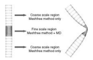
FIGURE 19.28 Multiscale analysis of carbon nanotube.
