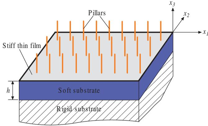
Fig. 1: (Color online) Schematic of periodic pillars adhered on a stiff thin film bonded to a soft substrate with thickness  $h$ .
