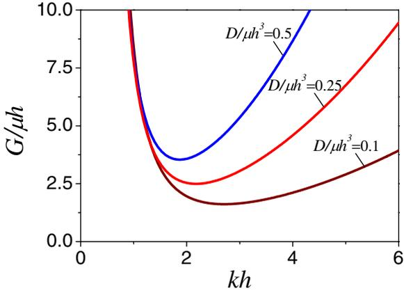
Fig. 2: (Color online) Variations of the dimensionless loading parameter  $G/\mu h$  with the wave number  $kh$  of the wrinkles, for several different bending stiffnesses of the thin film.
