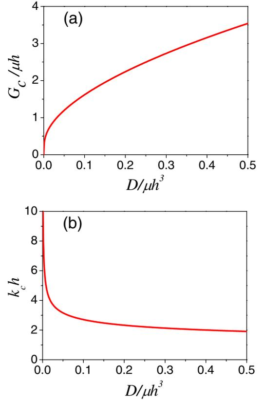
Fig. 3: (Color online) Variations of (a) the critical load  $G_c/\mu h$  for wrinkling the system and (b) the critical wave number of the wrinkles  $k_c h$  with the normalized bending stiffness of the thin film  $D/\mu h^3$ .
