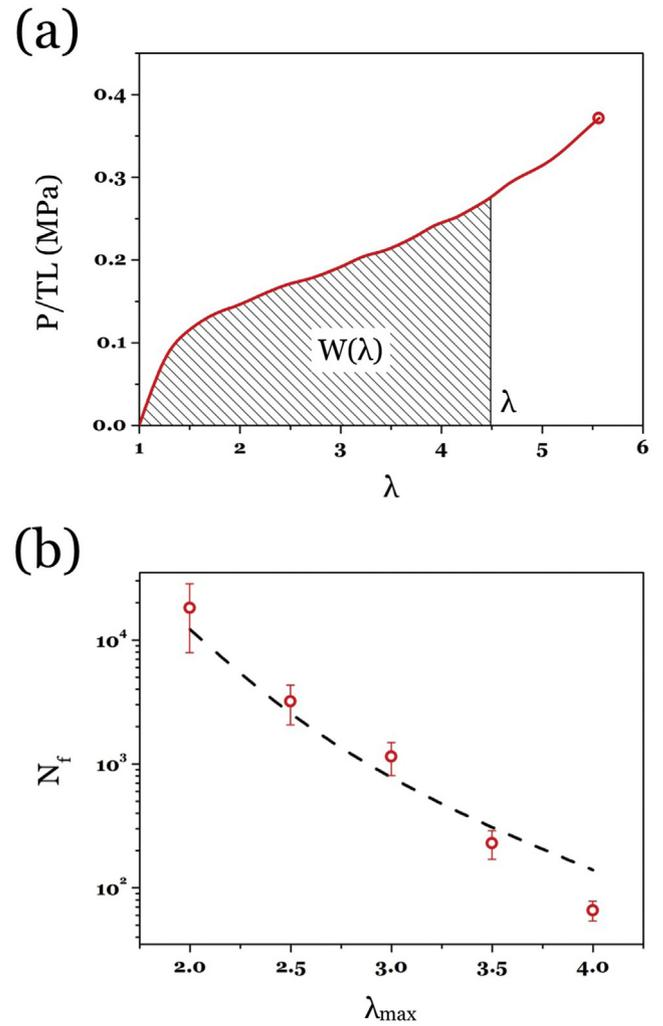
**Fig. 4.** (a) Measurement of strain energy for pristine VHB film under simple extension test; (b) Fatigue lifetime for VHB film with an edge crack with initial crack length  $c_0 = 1$  mm under cyclic loading-unloading simple extension test. The black dash line is prediction and red cycles are experimental measurements. (For interpretation of the references to colour in this figure legend, the reader is referred to the web version of this article.)
