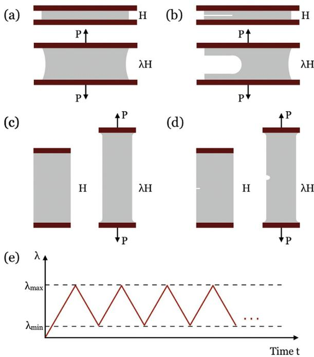
**Fig. 1.** Schematics of a VHB film subject to cyclic loading-unloading test. (a) A pristine VHB film under pure-shear test in undeformed state and deformed state; (b) A pre-cut VHB film under pure-shear test in undeformed state and deformed state; (c) Cyclic loading-unloading test with stretch rate: 1.8/s.
