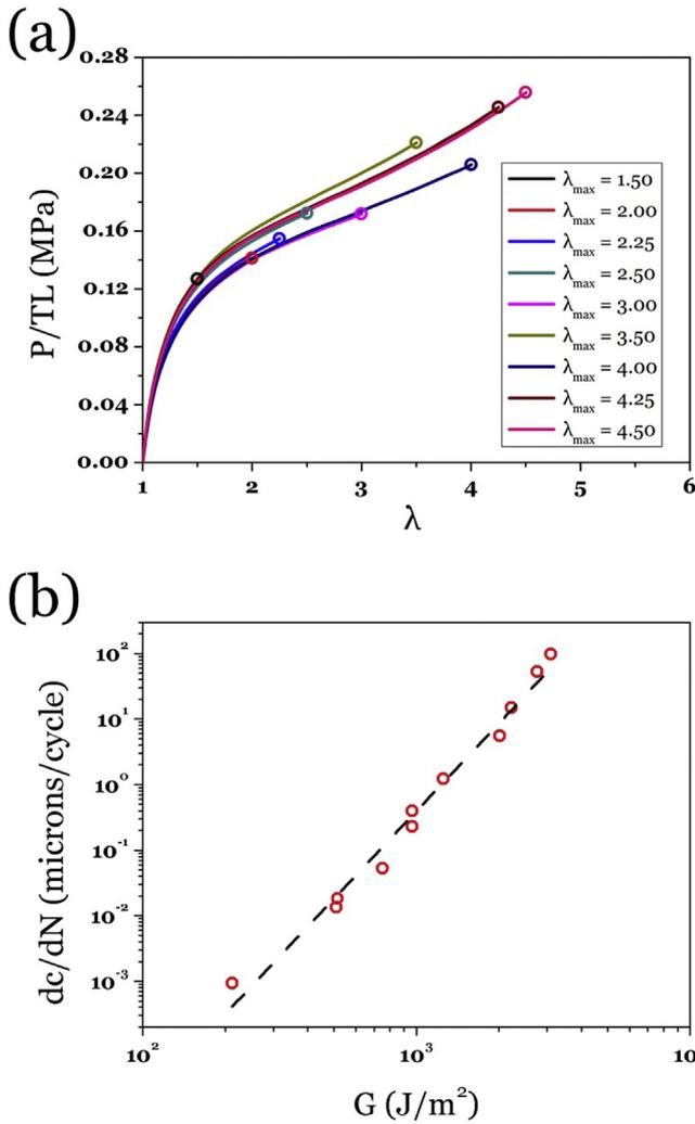
**Fig. 3.** (a) Stress-stretch curves of pristine VHB film subject to pure-shear test with different maximum stretches; (b) Dependence of crack growth rate on maximum energy release rate. Red cycles are experimental measurements. Black dash line is a fitting line. (For interpretation of the references to colour in this figure legend, the reader is referred to the web version of this article.)
